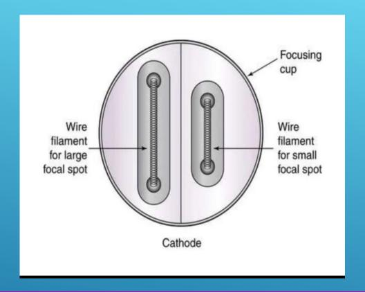
the large (2 cm) filament for large part, high exposure the small (1 cm )filament for small part, low exposure
