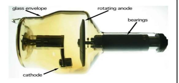
2. Establish a high voltage potential between the anode and cathode to accelerate the electrons.
